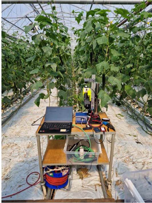
Figure 9. Measuring system collecting data in a cucumber greenhouse with powdery mildew attack.
